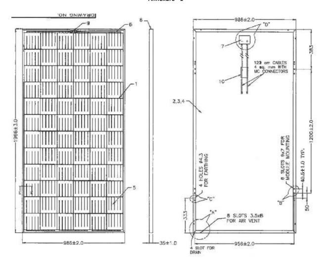
This is BHEL PV module drawing. Vendor to submit their PV Module drawing incorporating the mounting hole pitch of  $1200 \times 956$  mm.
